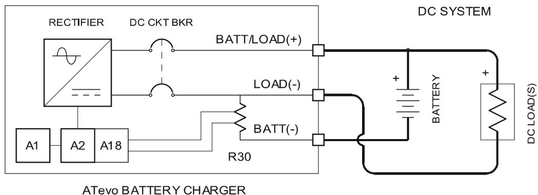
**NOTICE** Battery charge/discharge options are specifically designed for a one battery, one load, and one charger installation. See *Application Note* ([JD0052-00](#)) for utilizing shunt in a *dual* charger system.
