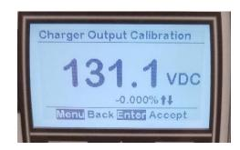
Does the ATevo meter reading (Vdc) match the external dc voltmeter?
