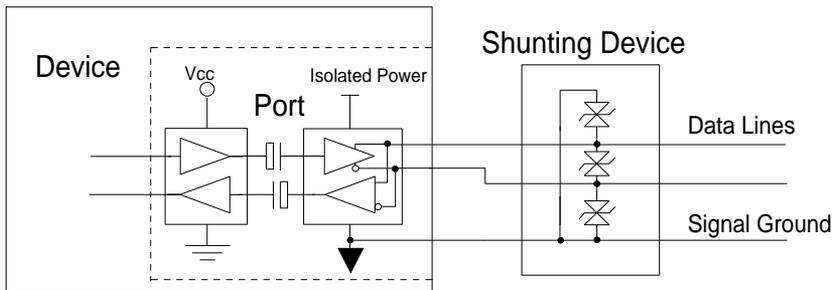
**Figure 4.8 Isolated port with ungrounded shunt protection**
